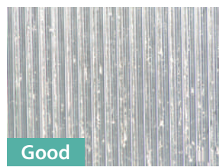
Cutting edge conditions comparison - after 40 min machining - (Internal evaluation)
