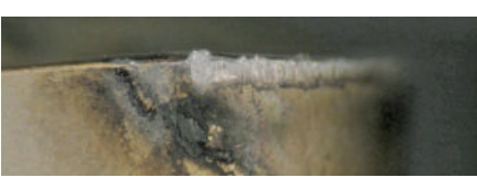
Cutting edge conditions comparison - after 40 min machining - (Internal evaluation)
