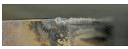
Cutting edge conditions comparison - after 40 min machining - (Internal evaluation)
