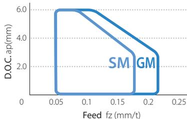
Cutting conditions :  $V_c = 150$  m/min,  $a_e = DC/2$  mm, Workpiece : S50C
