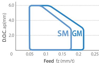
Cutting conditions :  $V_c = 150$  m/min,  $a_e = DC/4$  mm, Workpiece : S50C
