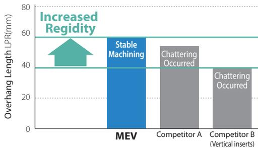
Cutting conditions : Vc = 200 m/min, ap x ae = 3 x 18 mm, fz = 0.10 mm/t, ø20 (3 inserts), Dry Workpiece : SCM440 (H)
