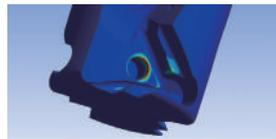
Prevents breakage from toolholder with decreased max. cutting stress
