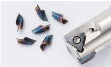
Cutting conditions :  $V_c = 150$  m/min,  $a_p = 6$  mm (Slotting),  $f_z = 0.2$  mm/t,  $\phi 20$  (3 insert), Dry Workpiece : S5400
