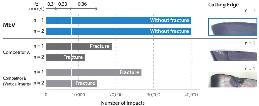
Cutting conditions :  $V_c = 120$  m/min,  $a_p \times a_e = 2 \times 10$  mm,  $f_z = 0.3 - 0.36$  mm/t,  $\phi 20$  (1 insert), Dry Workpiece : SCM440 (H) (37~39HS)
