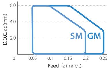
Cutting conditions :  $V_c = 150$  m/min,  $a_e = DC$  mm, Workpiece : S50C
