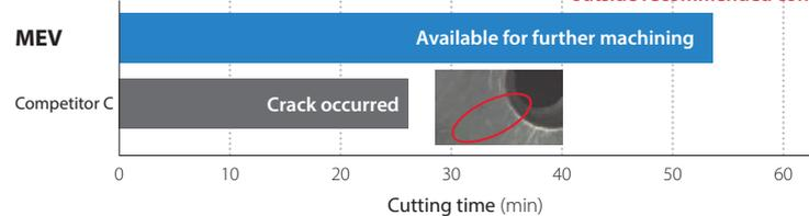
Cutting conditions : Vc = 120 m/min, ap x ae = 5 x 7.5 mm, fz = 0.25 mm/t, ø20 (1 insert), Dry Workpiece : SCM440 (H)
