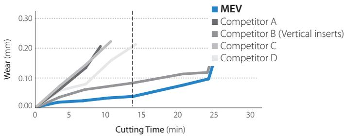
Cutting conditions :  $V_c = 180$  m/min,  $a_p \times a_e = 3 \times 10$  mm,  $f_z = 0.1$  mm/t,  $\phi 20$ , Dry Workpiece : SKD11 (30~35HS)
