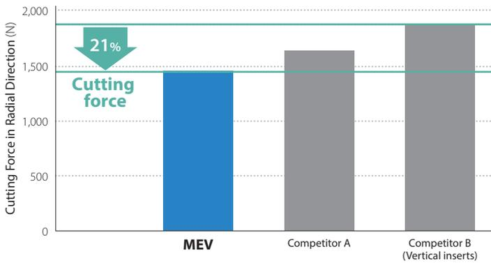
Cutting conditions : Vc = 200 m/min, ap x ae = 3 x 18 mm, fz = 0.10 mm/t, ø20 (3 inserts), Dry Workpiece : SCM440 (H)
