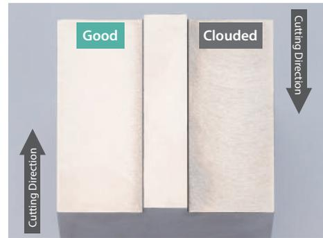
Cutting conditions : Vc = 180 m/min, ap x ae = 3 x 40mm, fz = 0.1 mm/t, ø50 (5 inserts), Dry Workpiece : S50C
