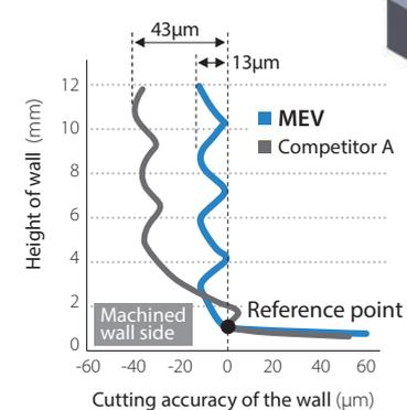
Cutting conditions : Vc = 200 m/min, ap x ae = 3 x 10mm (4 pass), fz = 0.15 mm/t, ø50 (5 inserts), Dry Workpiece : S50C
