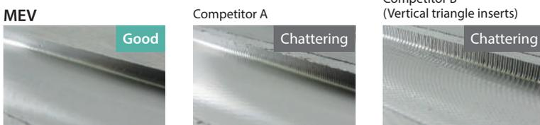
Cutting conditions : Vc = 220 m/min, ap = 3 mm (Slotting), fz = 0.10 mm/t, ø20 (3 inserts), Dry Workpiece : SCM440 (H)
